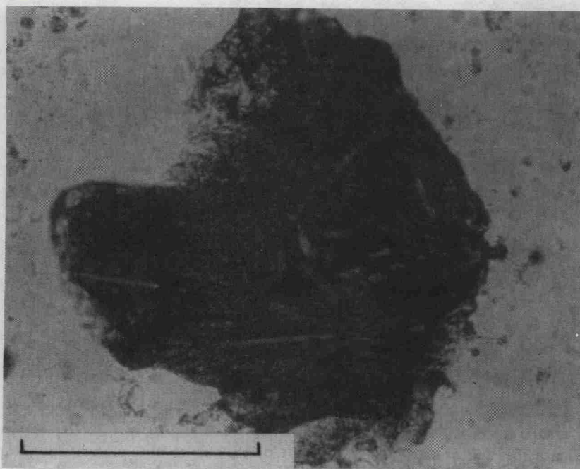
Figure 38. Dark reddish-brown fragment with well-developed quench crystals of pyroxene arranged in parallel and radiating arrays in a matrix of less crystallized glass. Fragment 318,510; plane polarized light; scale bar 0.1 mm.
